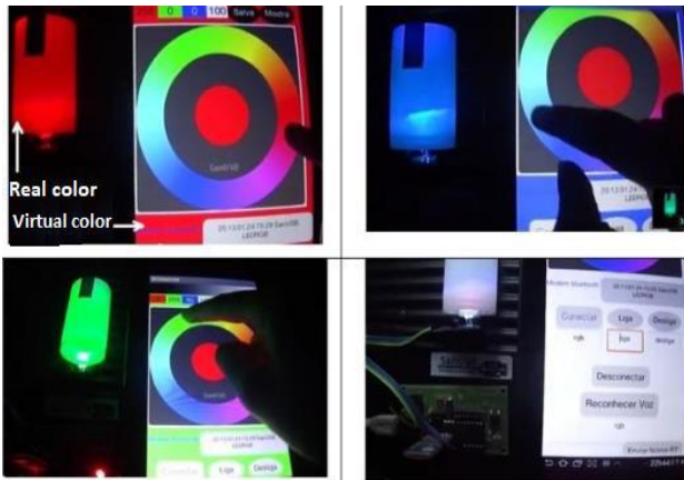
Fig 9: Operation of the BT4SanUSB app during formation of real colors on the RGB LED and virtually on the Android device
