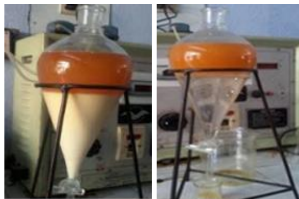
Fig. 4 Soaps separation Fig. 5 Clean water in washing
